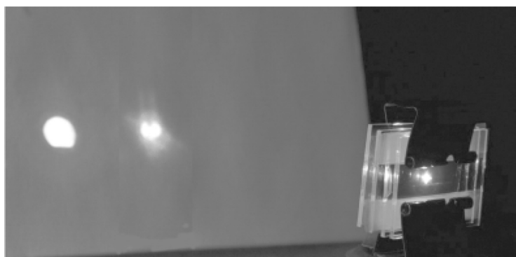
FIGURE 5 Laser emission from the sandwich cell.
